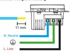
Wiring scheme for EK-PWS-UK-USB
