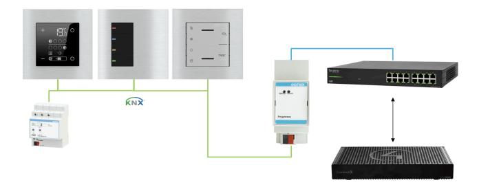
This specific functionality does not require any configuration in C4 TOOLBOX, and can be easily reached with a standard KNX communication driver offered by Control4, as better explained in the dedicated chapter "CONTROL4 INTEGRATION" in the following of this document.
