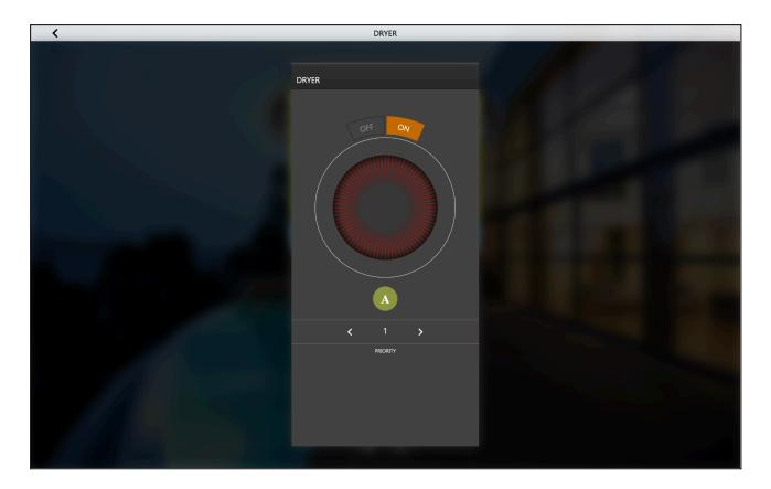
The top buttons offer the possibility to switch the load ON or OFF; in case of loads with integrated energy metering, the corresponding measurement is shown in the center part of the visualization.
