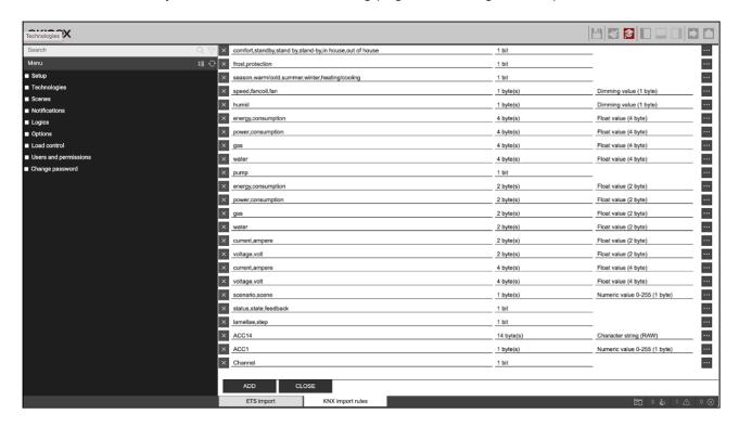
The rules look for one or more keywords within the group address names and automatically assign the correct data encoding (necessary for proper supervision) and the graphical appearance of the corresponding objects.
