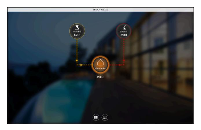
The orange colour highlights that the energy demand is partially "green"; the green colour is reached only in the event of production at least equal, or higher to the energy demand (and the excess energy is sent to the grid, and we talk of "immission"):
