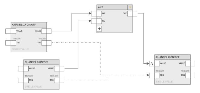
Please take care of the symbol in the input VALUE node, that switched to the TRIGGER symbol due to the fact that a trigger has been connected.
