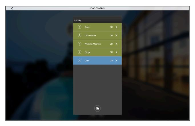
Each load is identified by a label, the actual priority and the current state (ON or OFF). By pressing the element, the following details are displayed:
