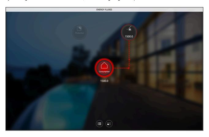
The graphic element in the center represents the real-time energy consumption of the building. If a production system is not available, the entire power demand is provided by the grid; in such a case, the symbol is in red color, meaning that no contribution is given to the power demand.
