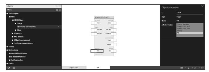
When selecting one or more nodes instead of the "all" wildcard predefined choices, only commands to those nodes will be forced when a trigger is received (in case of input nodes) or, as opposite, only upon a change of those nodes a trigger will be raised in case of output TRG.
