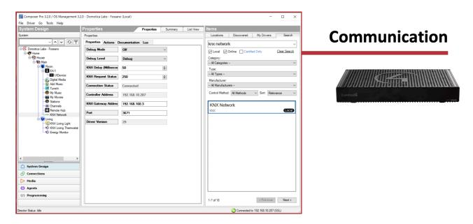
The IP address of C4 TOOLBOX must be entered in the KNX GATEWAY ADDRESS field; once entered, the driver attempts a connection and, if successful, updates the CONNECTION STATUS to CONNECTED.
