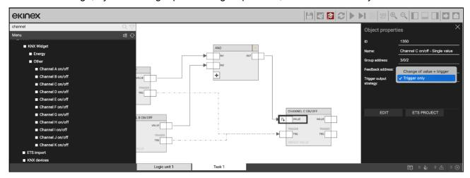
In the case of composite widgets, by opening the details (side panel) on the TRG node, it is possible to filter the nodes that determine the impulse (for input triggers) or that are influenced by the trigger (in output), through the multiple selector. The following pictures contains an example of multiple choice, when the TRG node is selected on a widget containing more than one sub-item:
