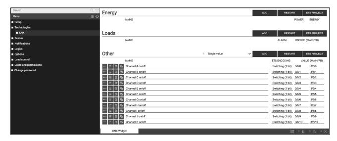
When changes to the KNX widgets configuration have been completed, press any occurrence of the RESTART button in order for the communication driver to make them operative.
