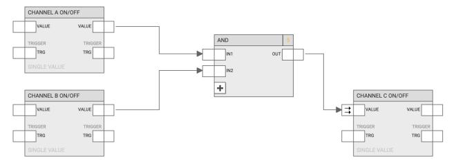
... the state of the KNX widget "Channel C" is kept aligned with the AND between the states of "Channel A" and "Channel B".
