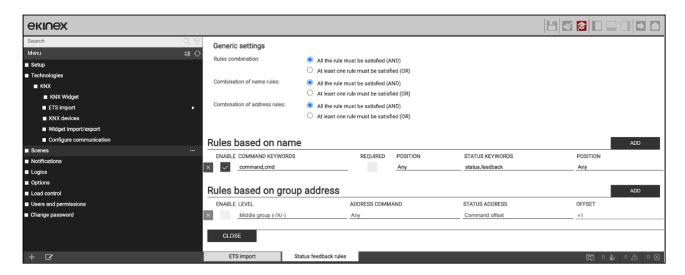
The correct configuration of these rules is very important, in order to greatly speed up the subsequent work of configuring widgets. If C4 TOOLBOX is not correctly instructed on the relationship between command and feedback addresses, in fact, it cannot pre-compile the selection of these address pairs when creating a new widget.
