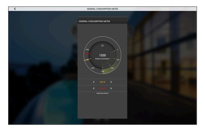
As soon as the higher limit is reached (red colour) the load control starts switching off the loads; the restore back to normal functioning of the loads does not happen until the energy demand goes under the lower limit (yellow colour). As long as the power demand keeps between the two limits, the situation continues to be monitored by the system, but no action is taken on the loads.
