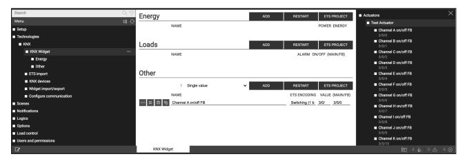
The imported group addresses can be drag & dropped into the MAIN and FB fields; it is suggested to start with the main (command) address. If the command-status rules have been properly configured during the ETS import process, the status feedback is automatically filled as soon as a command address is dropped.
