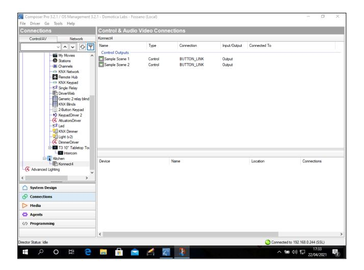
These connections can be bound to other drivers, by offering in this way the possibility to execute the corresponding scene, each time an ON is received on the connection itself. The BUTTON\_LINK connection typology is best suited for push buttons, but can be normally associated with other ON/OFF connections available for the majority of drivers.
