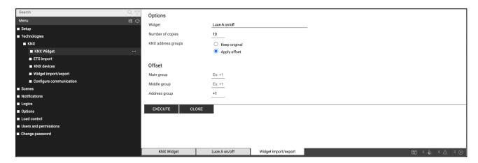
The number of widgets and the offset criteria for the automatic duplicate procedure can be entered, in the form of an offset (positive or negative) for each token of the three-level KNX addresses.
