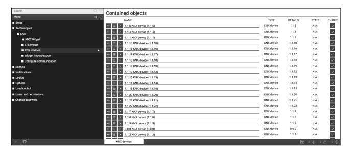
If a specific device must be excluded from the control, the corresponding ENABLE flag must be de-flagged. In order these changes to enter in action, when done, the communication services must be restarted in the
