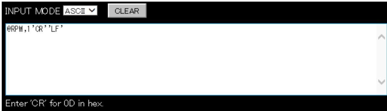
[Figure 9.24] Control command input box for ASCII
