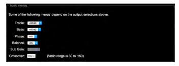
Values set here will be used by the 251 after power up. They can be adjusted at run time and stored (via the Automation Interface).
