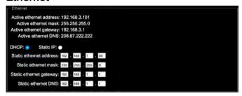
Allows you to change the Ethernet configuration. Note that incorrect settings may make the 251 unreachable via the web page.
