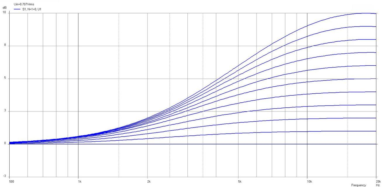
Note: Screen made with acoustically transparent fabric will have little impact (1 to 1.5 dB) in the upper frequencies. Micro perforated screen will have a stronger impact on the frequency response over 1 kHz.
