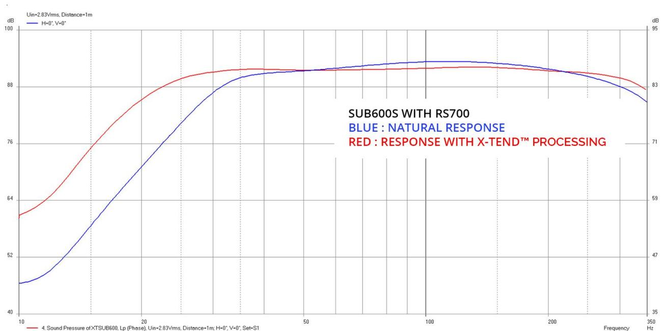
**Note:** X-TEND™ processing provides more extension and works simultaneously with X-GUARD. It has been optimized for SUB600S only. Depending of the signal profile at extremely low frequencies max SPL might be reduced in some cases.
