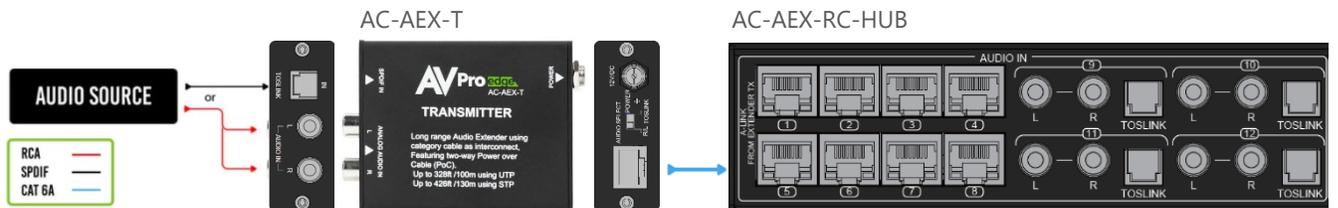
**⚠ IMPORTANT:** Each A-LINK port on the AC-AEX-RC-HUB must be paired with an AC-AEX-T audio extender transmitter for complete operation.
